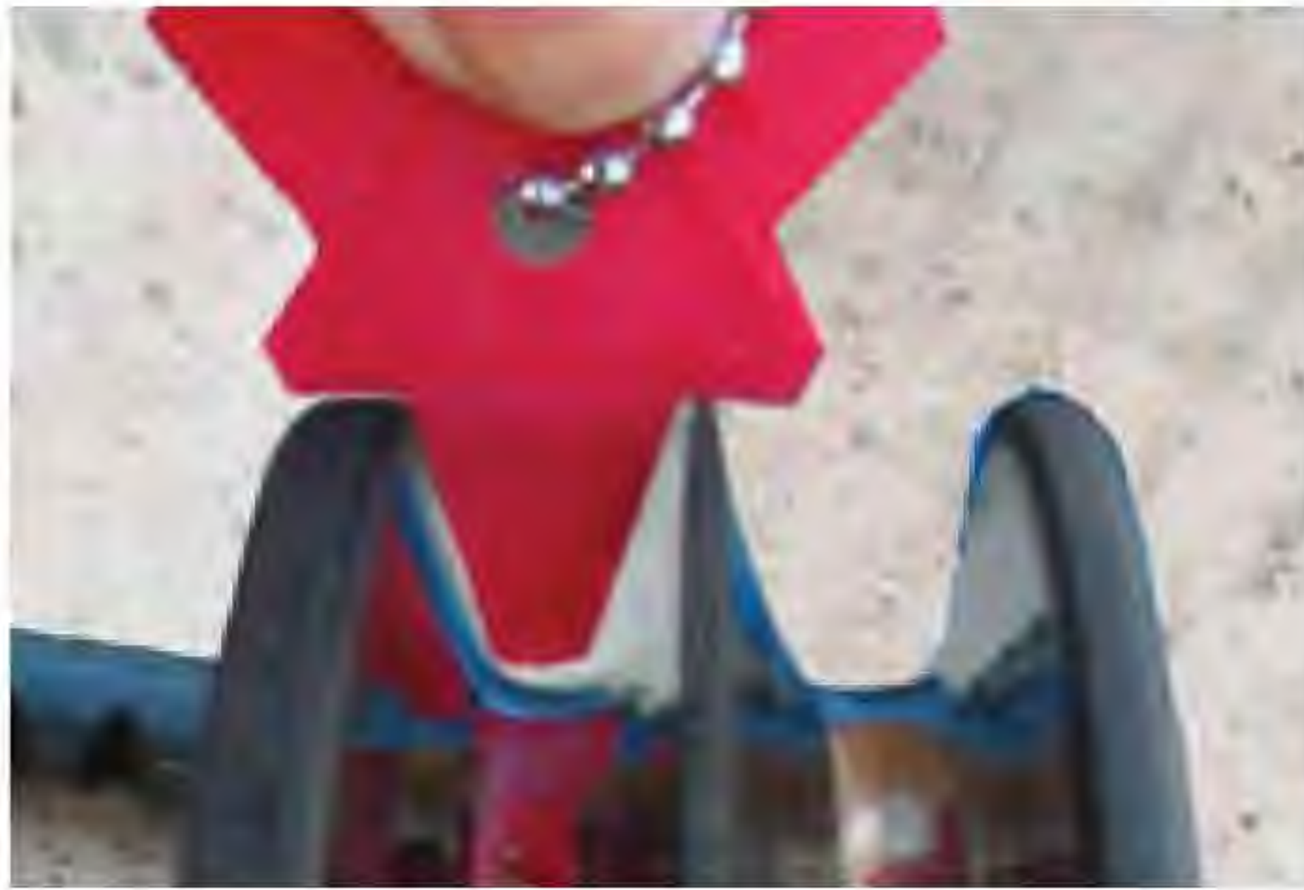
Figure 20 - An investigation into a customer's belt failure complaint identified this severely worn sheave.
