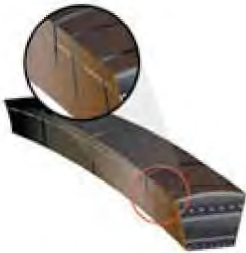
Figure 14 - Belt surface hard or stiff
