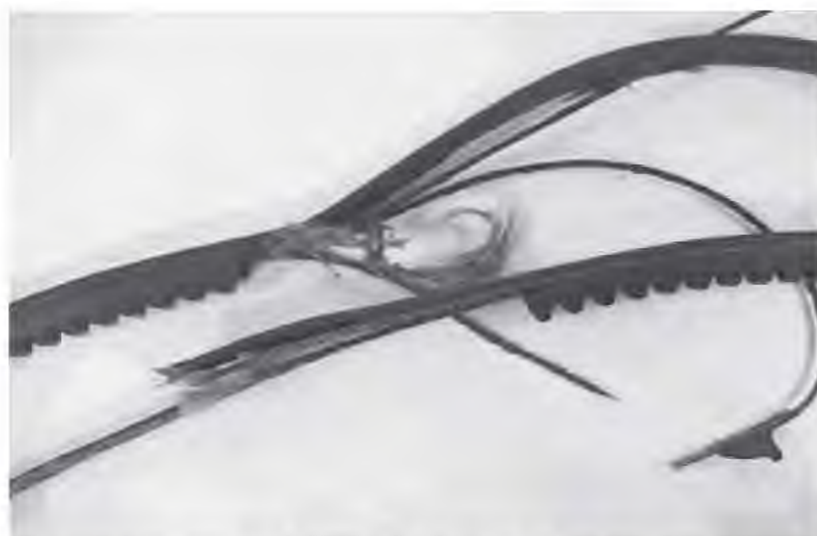
Figure 1 - Normal V-belt failure is characterized by a break or separation.
